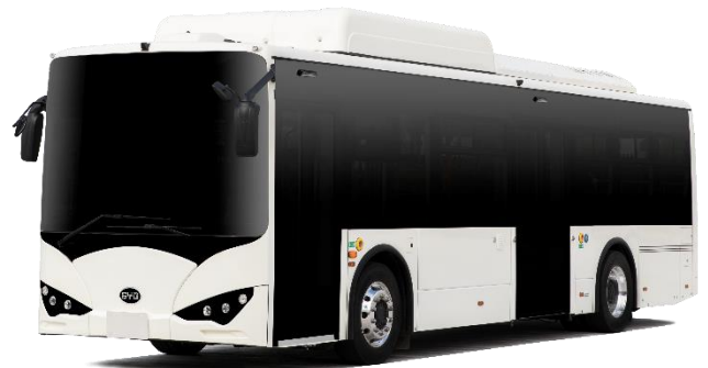
Large electric bus "K8"/Vehicle length 10.5m/ Approx. 220 km cruising range
