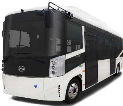
Small electric bus "J6"/Vehicle length 6.99m/Approx. 200 km cruising range
